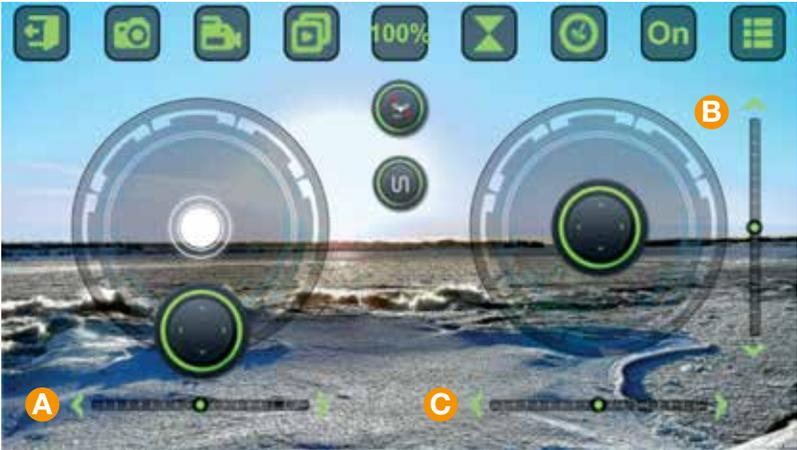
To calibrate the drone back to normal settings, use the Trim settings found below the left and right throttle stick, icons.
